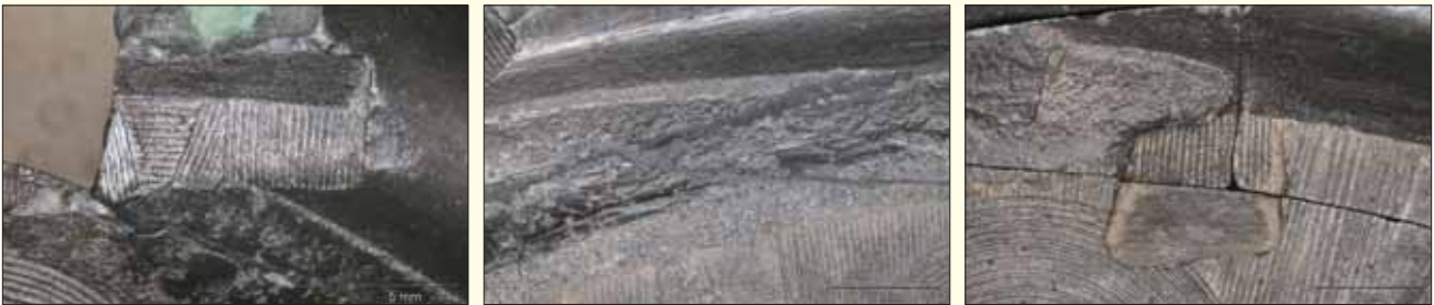
(1) Defect containing design (Defect 1) (2) Corner scab defect (Defect 2) (3) Defect containing design (Defect 3)
