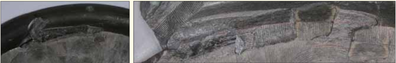
(7) Location of Casting defects 1, 2, 3 (8) Original position of Casting defects 1 and 3
