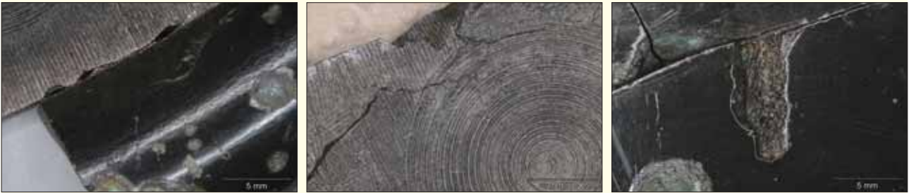
(4) Rat-tail defect and scab on the lower part of the outer section and rim (5) Casting defect located on the upper part of the back of the mirror (6) Casting defect located on the upper part of the front of the mirror
