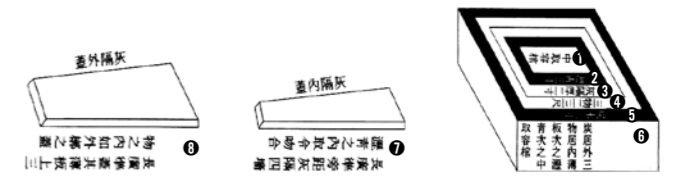
Fig. 1. Schematic plan of a lime mortar structure and the inner and outer covers (築灰隔及内外蓋圖, Chukhoigyuk geup naeogae do ): ① gwan (棺, burial compartment), ② yeokcheong (瀝青, presumed to be an oily mixture, but not yet identified through archaeological investigation), ③ hoegyek (灰隔, wooden cist structure) ④ sammul (三物, packed lime mortar mixture), ⑤ sut (charcoal mixture), ⑥ explanation of structure, and ⑦ and ⑧ cover. (Illustration Volume of Commentaries on the Various Theories Concerning the Family Rituals of Master Zhu)
