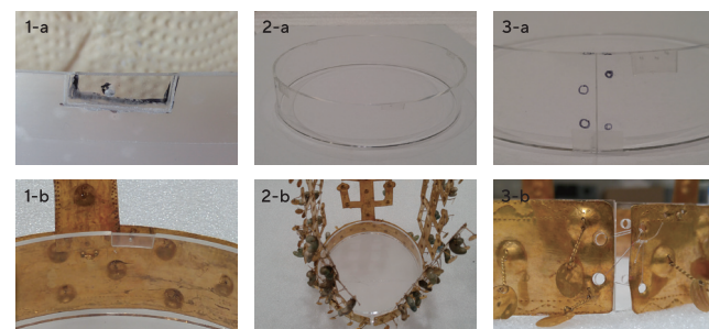
Fig. 14. The process of manufacturing the acrylic support 1) section affixing the dome-shaped decoration 2) the acrylic headband positioned within the gold crown 3) identifying the locations of the holes for affixing the headband prior to and after boring the holes
