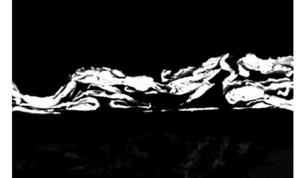
Fig. 52. Cross-section of the lacquer around the gilt designs 2 (SEM).
