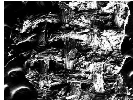
Fig. 35. Weaving of the fabric base (SEM of the backside of the lacquer layer).
