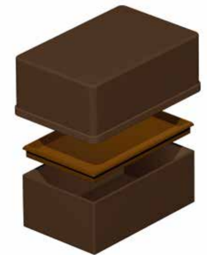
Fig. 1. Three-dimensional diagram of the incense box (from the top: cover, inner tray, and inner box).
